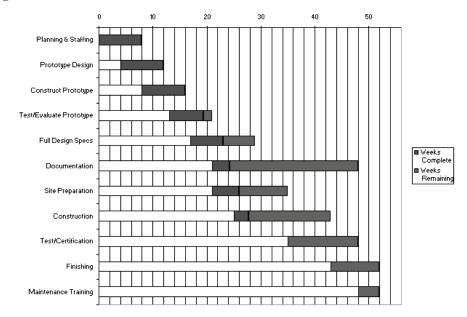
The Excel chart wizard was used to create Figure 15.2 with the columns for task, start week, weeks complete, and weeks remaining; the first part of each bar was made the same color as the chart background (the chart is shown in black and white here, but the completed and remaining parts of each bar are different in color). There are also spreadsheet templates available from a number of sources to facilitate Gantt-chart creation.
