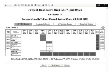
Figure 15.11 is a screen print from the FiveAndDime system of a rollup to the top level of a WBS showing progress (percentage complete), plan costs, actual costs, and earned value.
